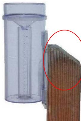
**Bevel** the top of the post to reduce rain splashing into the gauge.
