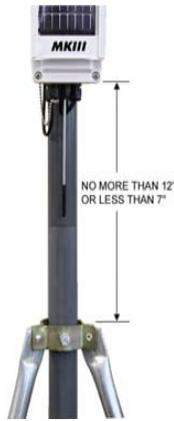
1. Mount the support tube as indicated above. Insert the necked down end into the **MKIII** sensor assembly, until it bottoms with the retaining screw in the slot. Tighten the screw.
