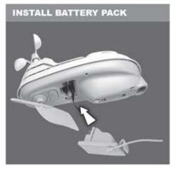
Install the wired battery compartment cover into the 5-in-1 Sensor.
