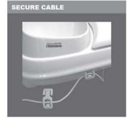
6. To further secure the wired battery compartment cover to the 5-in-1 Sensor, insert the three (3) in-line clips into the 5-in-1 Sensor as shown. The cord must be taut along the base of the sensor to prevent it from interfering with the sensor's wind vane.
