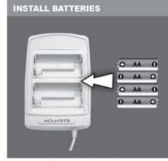
Insert 4 x AA alkaline or lithium\* batteries into the battery compartment. Heavy duty or rechargeable batteries are not recommended.
