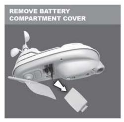
Remove battery compartment cover from the bottom of the 5-in-1 Sensor (keep or discard). Remove batteries if currently installed.
