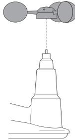
Tighten set screw with Allen wrench.
