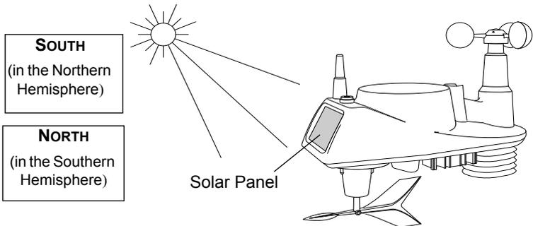
**Note:** If you install the ISS with the solar panel pointing in a direction other than south, you will need to use the wind direction calibration function in the Vantage Vue console in order to obtain accurate wind direction readings. See *Vantage Vue Console Manual* for more information.
