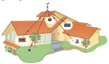
This illustration shows the **MK III** mounted on a remote building with the integral-mounted rain gauge. The **MK III** can be located on any convenient remote support as long as it is in range of the receivers. Preferably, the **MK III** should be higher than the receivers
